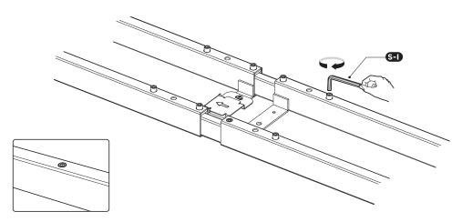
Retighten all the hex head screws to finish the adjustment.
