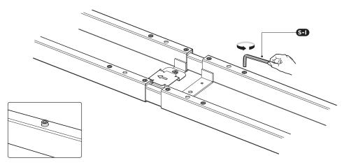
Loosen the hex head screws that fix the adjustable junction, but don't completely take out the screws.
