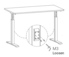
Loosen the screws at the adjustment protection.
