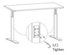
Tighten the screws at the adjustment protection again.
